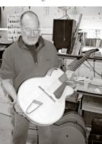
up where the string break angles over the bridge and the headstock are low and the string length tends to be long beyond them. I'm using a 25.5" scale because I really believe in it, and the guitars are very easy to play. Also, because of the adjustable neck joint, you can lower the action so it plays like an electric, or raise it and play slide, and you don't have to re-tune.
